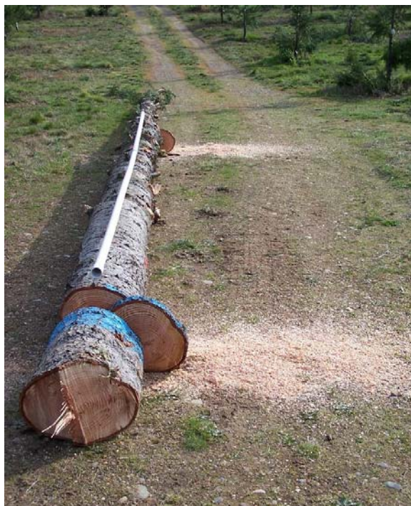
Figure 4. Removing wood disks from both ends of a butt log (17' log cut above the graft union) at the Hood Canal Seed Orchard.
