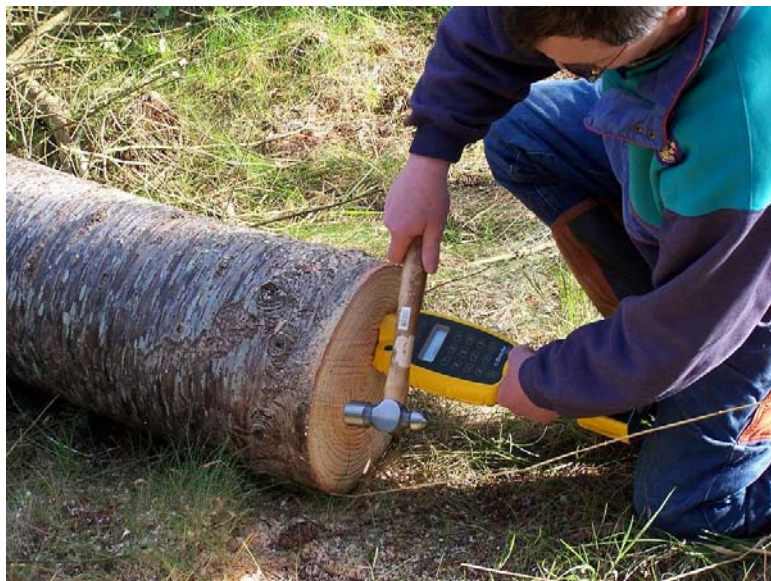
Figure 6. Measuring acoustic velocity of each log at the Hood Canal Seed Orchard.
